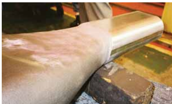
22. Portion of connection to be inserted.
