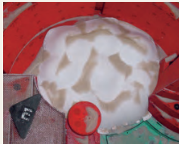
29. Snow drift modelling in water flume.
