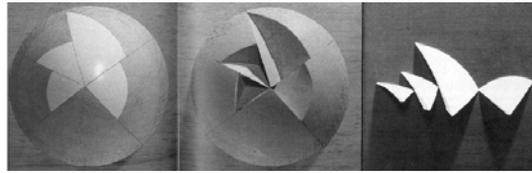
Figure A.76: Presentation of the spherical solution
