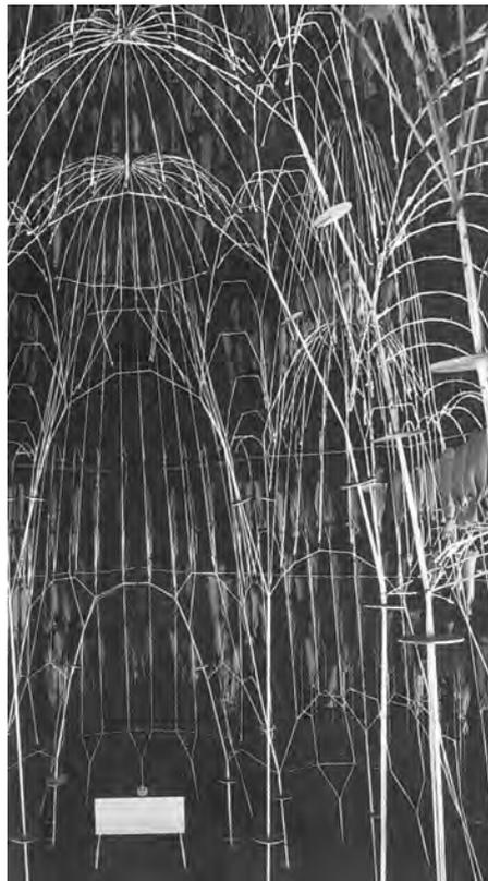
Figure 2.131: Reconstruction of hanging model from Gaudí. Image from (K. Bach 1988).
