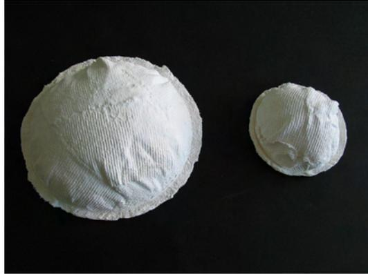
Figure 2.83: Inverted hanging cloth model, strengthened with plaster. Models by P.C. van Hennik.
