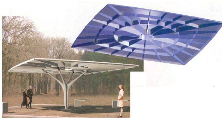
Figure A.81: The roof of the shed is 25mm thick and the stiffening ribs are 40mm thick
