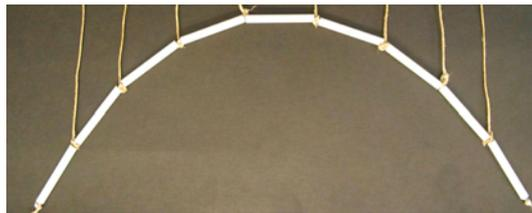
Figure 2.71: Hanging chain model upside down to find the pressure shape.
