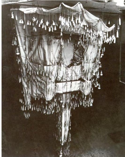
Figure 2.68: Hanging model by Gaudí. Image from (i Armengol 2001).
