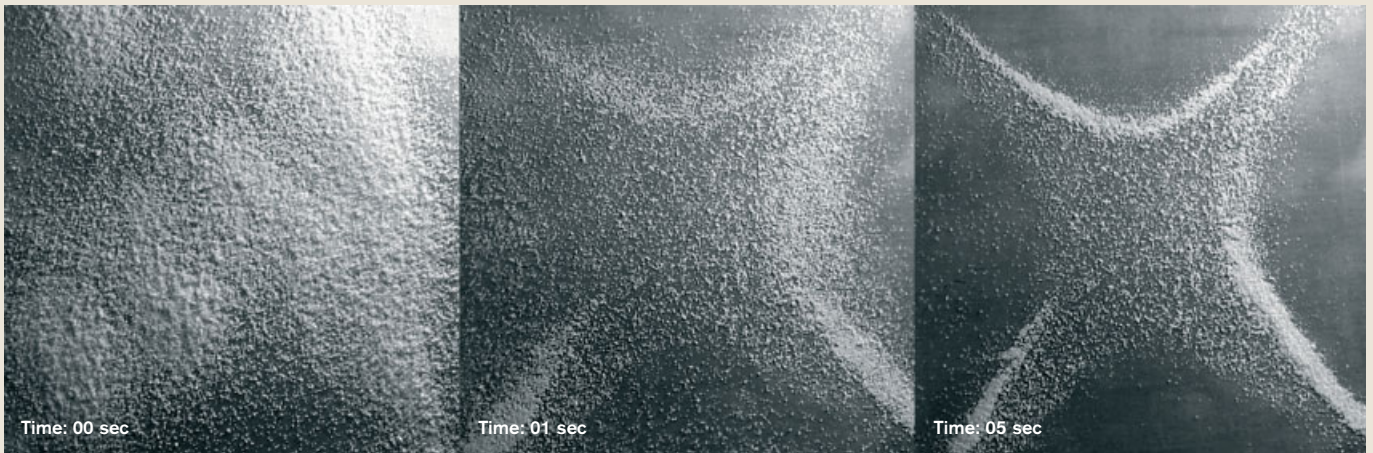
The image sequence shows a sand formation under the influence of frequency over a period of 6 seconds (from left to right).
