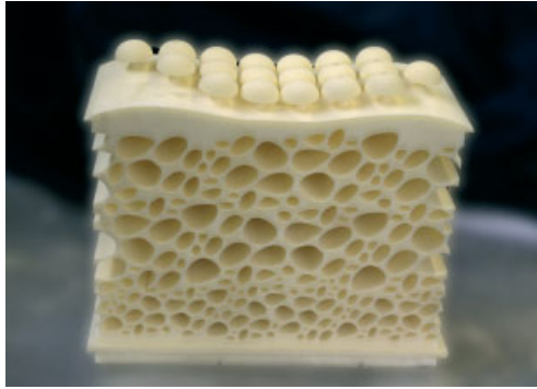
Single-material structure printed by selective laser sintering (SLS) and showing the freeform curvature of the surface.
