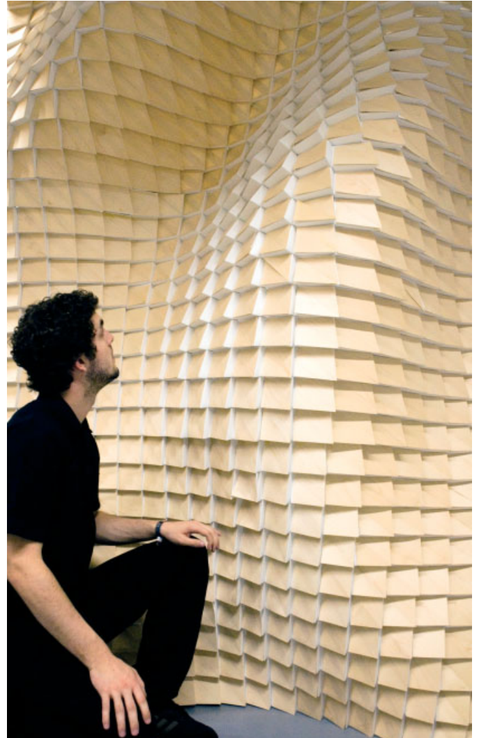
Assembled from more than 600 geometrically different veneer composite components, the full-scale prototype is both structure and responsive skin.
