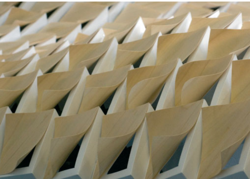
Responsive surface structure that instrumentalises moisture-content activated shape changes of timber components. See 'Material Performance' on page 34.
