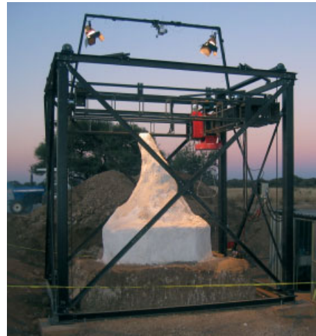
Large-scale digital slice and scanning apparatus as used in Namibia in August 2006 to slice 1 millimetre (0.04 inches) at a time from the mound. The exposed top face is then digitally scanned, generating thousands of scan images of the internal geometry of the actual mound.
