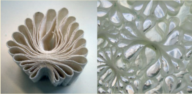
A glass-fibre band manipulated through a parametric gathering technique is the basic component (left) within a larger composite surface structure (right).
