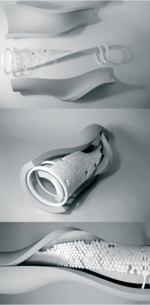
Preparation of a functional model at scale 1:20 to investigate specific assembly methods, induced displacement of the slender rods in buckling once bricks are incrementally added, and the overall behaviour of the assembly. A complex double-curved arrangement was chosen that comprises both positive and negative Gaussian curvature. A formwork was milled on a 5-axis CNC-router and bricks were rapid prototyped (selective laser sintering). The slender rods were fixed at the end positions and the bricks incrementally assembled. In this process the rods undergo torsional buckling and the bricks receive compressive stress. In this way the system self-organises and self-stabilises, reducing the need for a full formwork during the assembly process.
