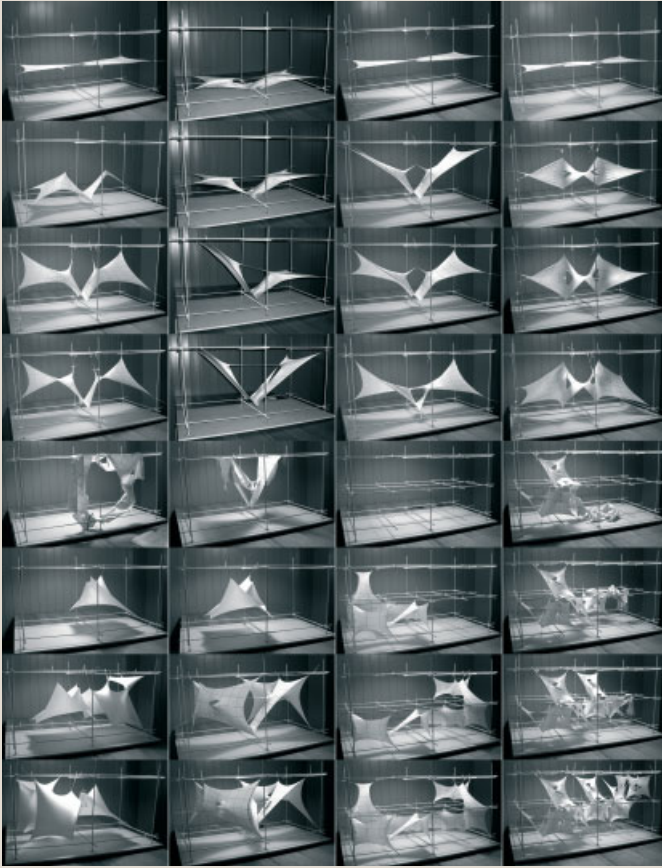
The physical form-finding of eight different membrane component and connection types (eight columns of four images each, from left to right and top to bottom) indicates different component proliferation possibilities.
